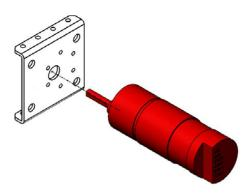
**Step 2**: Install six M3 x 0.5 x 6mm long socket head screws (am-1254) in each NeveRest motor to secure it to the gearbox plate
