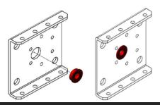
NOTE: Make sure the flange of the bearing is flush against the sheet metal of the gearbox plate.
