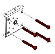
**Step 7**: Insert the Axle of the Gearbox Assembly into the bearing on the PicoBox Solo gearbox plate. Align the four 1/4-20 screws with the 1/4" holes on the PicoBox Solo gearbox plate.
